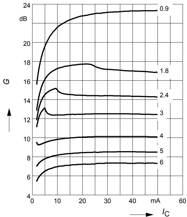
**Power gain  $G_{ma}$ ,  $G_{ms} = f(V_{CE})$**
